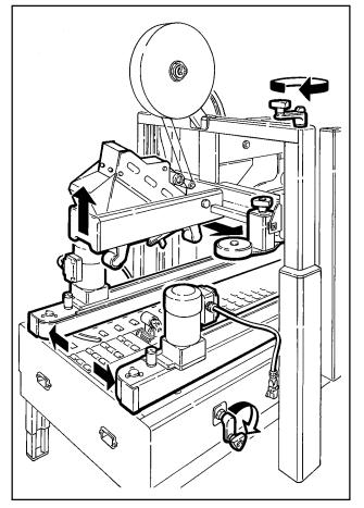
Figure 3-6 – Box Size Set-Up
